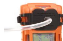
Bump/calibration plate To apply test gas to T4
